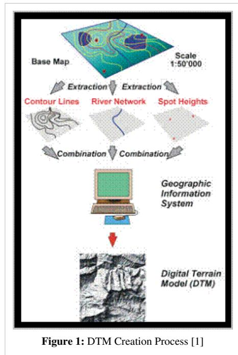
Figure 1: DTM Creation Process [1]
